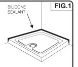
Once the walls have been tiled but **before** the enclosure is installed, the tiles **must** be silicone sealed to the tray all of the way around in one continuous bead.
