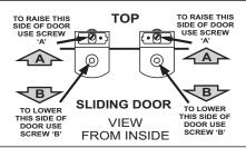
A Roller bearing adjustment- using screwdriver, loosen screw (do not remove), reposition in slot and re-tighten.
