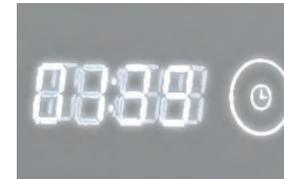
**Clock:** To operate, cover the sensor zone by moving your finger over it and press gently.
