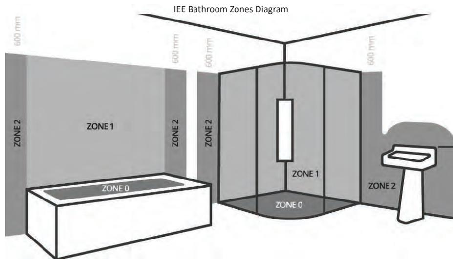
Bathroom fittings are subject to the appropriate zones in accordance with IEE Regulations. This product is **only** suitable for permanent indoor installation in **Zone 2** and outside zones. (See above) This product is **not** suitable for installation in **Zone 0** or **1**, saunas, steam rooms or shower cubicles. Do **not** connect to a trailing plug and socket. Do **not** install onto surfaces that are either damp or electrically conductive.
