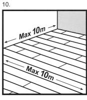
Maximum area of coverage without an expansion break is 10m x 10m.
