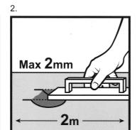
Prepare the subfloor, removing debris and ensuring it is level.
