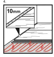
Expansion gaps must be 10mm minimum where UFH is in use.
