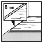
Expansion gaps of 6mm minimum are required around the perimeter of the room and around any fixed objects.
