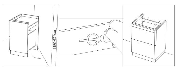
It is recommended that the unit and basin are secured to a suitably reinforced wall to ensure stability. This should be done using the wall hanging plates supplied. The wall fixings supplied are intended to be used on a solid brick walls. Check suitability before continuing.
