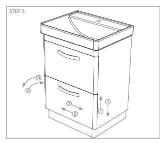
To make adjustment 1 (Up and Down) turn screw A (see Step 4) To make adjustment 2 (Left and Right) turn screw B (see Step 4)
