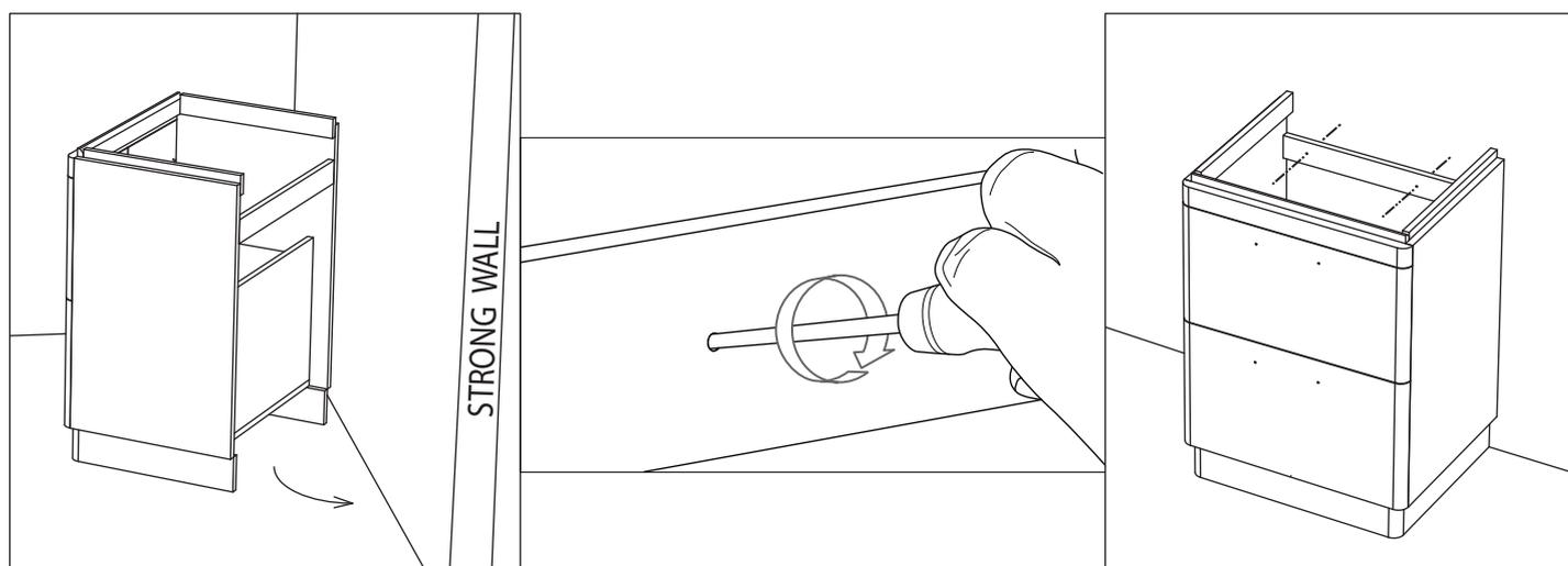
It is recommended that the unit and basin are secured to a suitably reinforced wall to ensure stability. This should be done using the wall hanging plates supplied. The wall fixings supplied are intended to be used on a solid brick walls. Check suitability before continuing.
